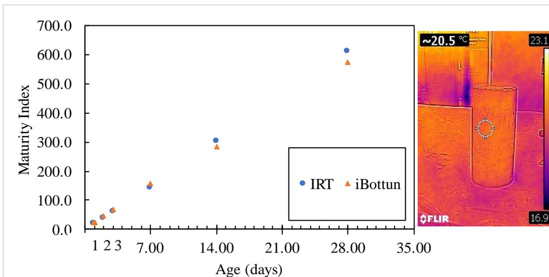
**Fig. 3:** Comparison of maturity index calculated from iButton and infrared thermography, IRT.
