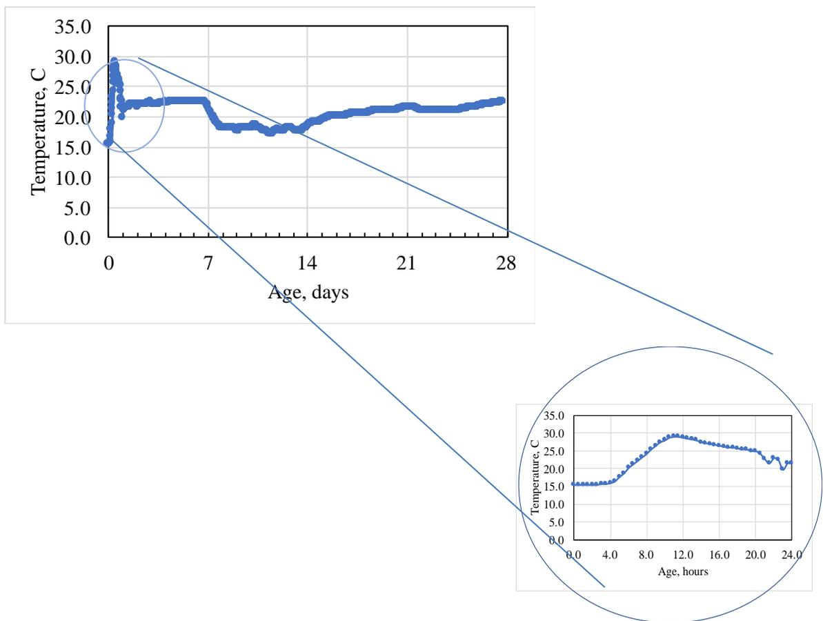
**Fig. 1:** Time-Temperature history of concrete during hydration.
