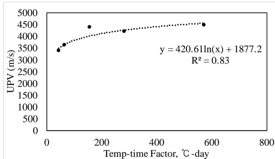
**Fig.4:**Relationship between UPV and time-temperature factor.
