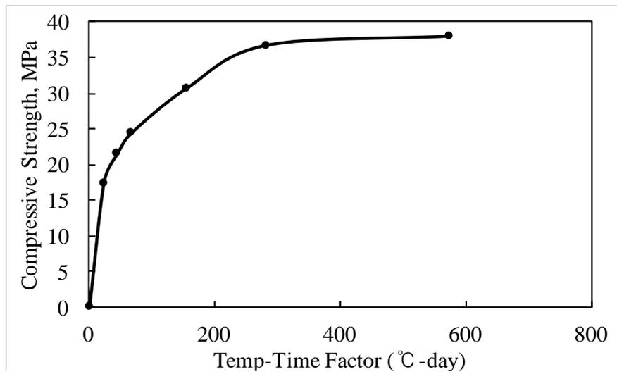
**Fig.2:** Compressive strength versus time-temperature factor during 28 days of curing
