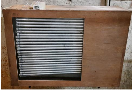
Figure 8: Waste Heat Recovery System
