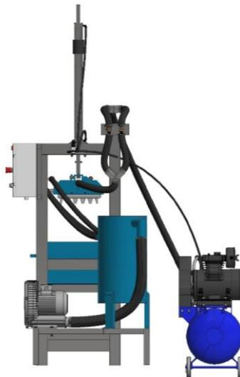
**Figure 3: Egg Tray Molding Machine Design (Right View)**
