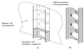
Figure 1 Cross Section of Castellated Column.
