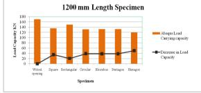
Figure 18 Decrease in 1200 mm Length Of Specimen
