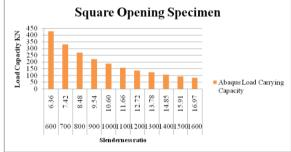
Figure 6 Castellated Steel Column With Square Opening
