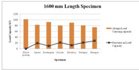
Figure 22 Decrease in 1600 mm Length Of Specimen
