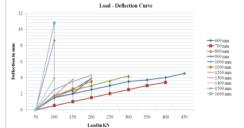
Figure 28 Load Deflection Curve for Tapered Shape with Pentagon Openings
