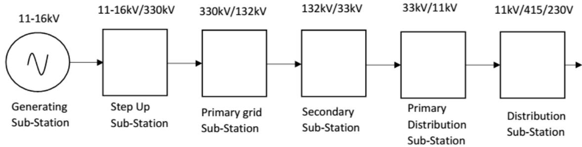
Figure 1: Electric Power Structure
