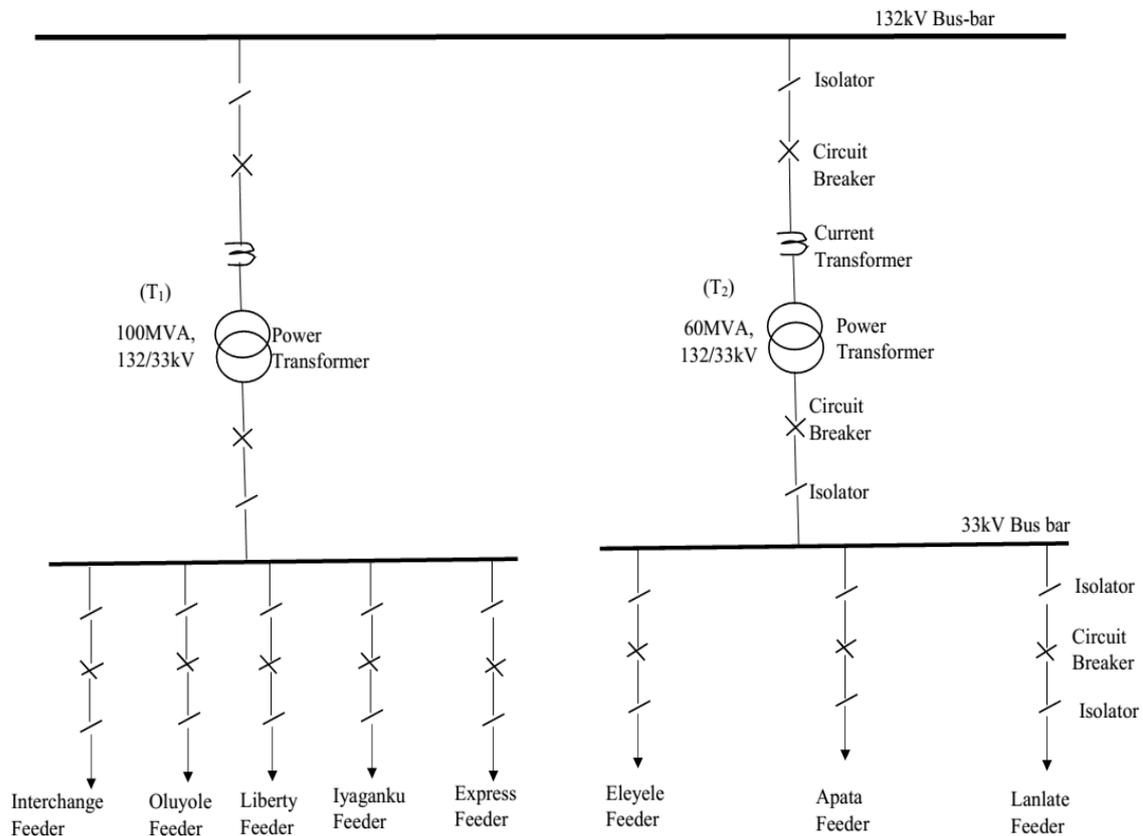
Figure 2: Schematic Diagram of Ayede 132/33kV Transmission Sub-station
