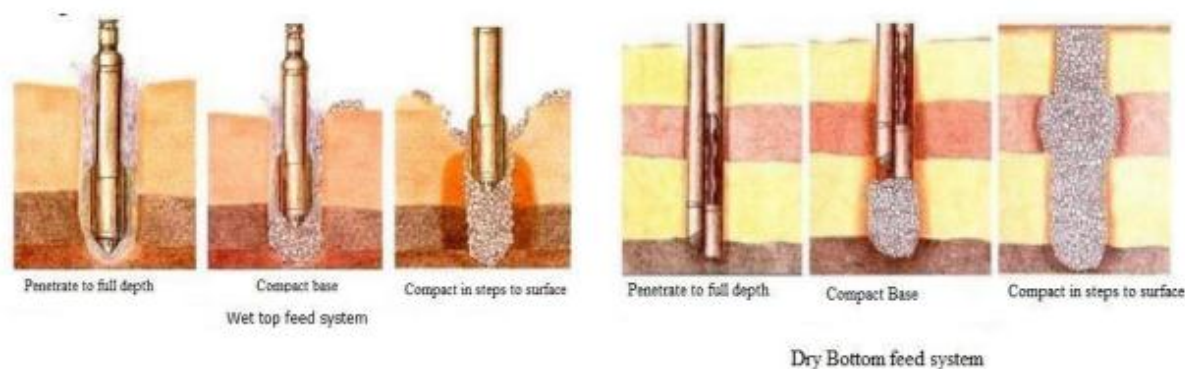
Figure 2: Jet Common used methods of stone column technique
