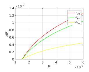
As the graphic shows, There is no shear initially, all three shears record the value zero. When the radius begins to grow, the shear rate found for the Diouf-Zidi model grows faster followed by the shear of the Knowles-Sternberg model with a difference which becomes biger and biger when the radius increases, this difference is in the order of 0.2 for radius of  $6 \times 10^{-3}$  between these both model.
