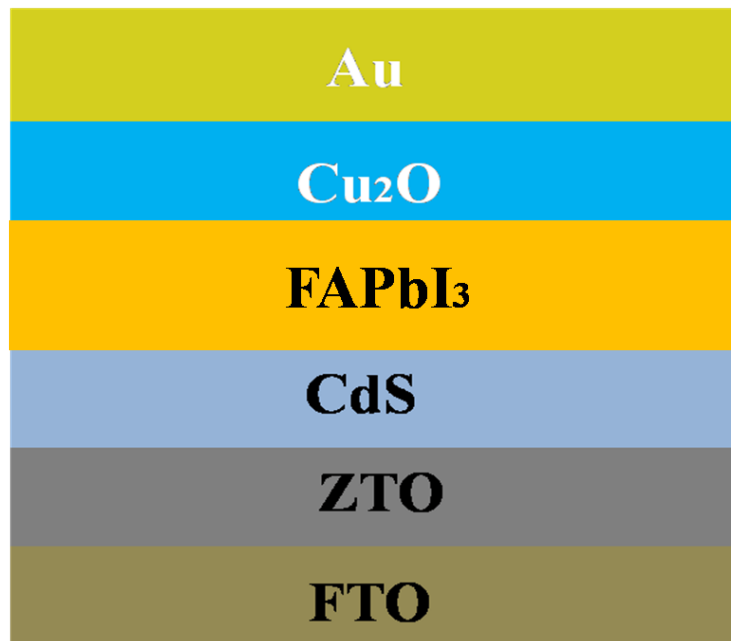
Fig.1: Cell configuration for simulated thin film solar cell
