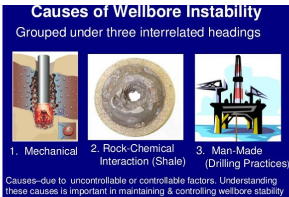
Figure 3: causes of wellbore instability Source: Bowling, (2012).
