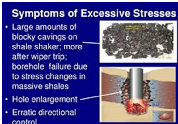
Figure 4: symptoms of excessive stresses Source: Bowling, (2012).
