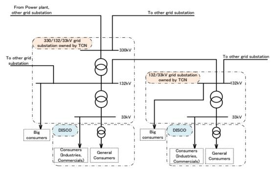
Figure 1. Structure of Transmission System (Japan International Cooperation Agency, 2020)
