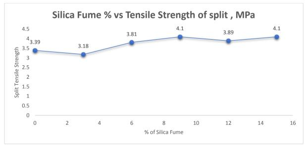
Figure: Split tensile strength at different percentages of silica fume
