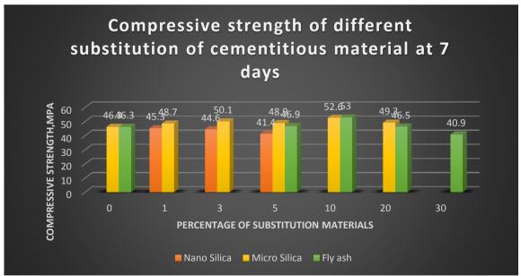
Fig: compressive strength of different substitutions of cementitious material at 7 days
