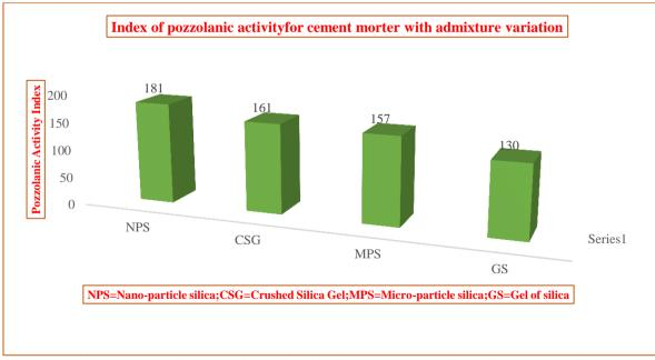
Figure: Index of pozzolanic activity for Cement Mortar with admixtures variation
