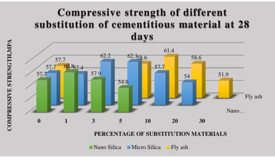
Figure: compressive strength of different substitutions of cementitious material at 28 days
