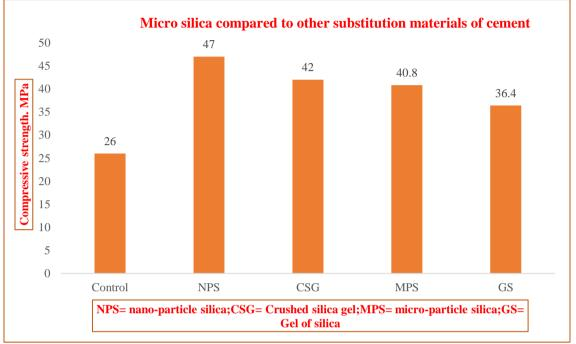
Figure: Compressive strength for cement mortar with different mixtures
