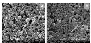
Figure: MS particles micrograph in un-compacted condition (a), compacted condition (b) (Soomro et al., 2023) MS is primarily grey, but it can range from nearly white to nearly black. Its surface area is between 15000-25000  $m^2/kg$ . MS particle tends to form agglomerations that are bonded loosely together (Fidjestol & Lewis, 1998).
