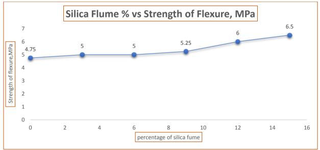
Figure: Strength of Flexure at different percentages of silica flume at 28 days
