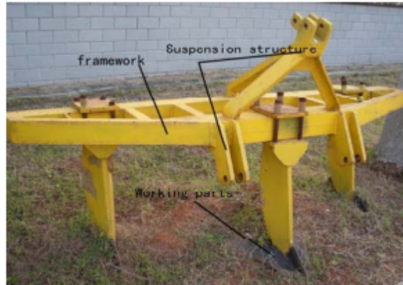
Figure 11: Structure of the 4UMS cassava harvester(Yuan zhang et al.,2011).
