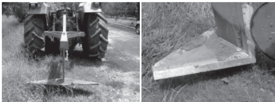
Figure 10:Prototype of a cassava harvester with a rigid V-shaped blade (Bernardo ospina et al.,2002)
