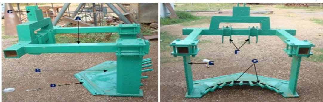
A – Beam to which digging unit is attached B – Conical mouldboard C – Top link hitching point D – Digger E - Vertical support F – Lower link hitching points G – Slatted rods for shaking off soil.
