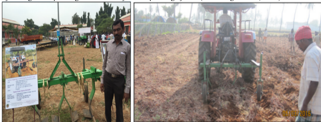
Figure 18: Demonstration of tractor operated cassava harvester (Velmurugan et al. , 2020).
