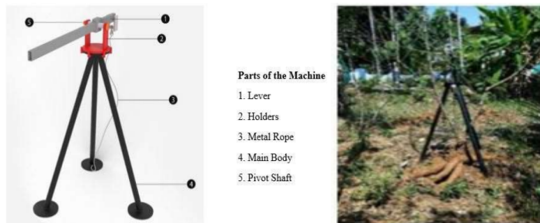
Figure 4:Catia design of the product and field testing(Aby Cherian,2018)
