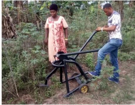
Figure 2:Field trial to showcase the operation of the semi-manual cassava harvester(Otonocha et al.,2021).
