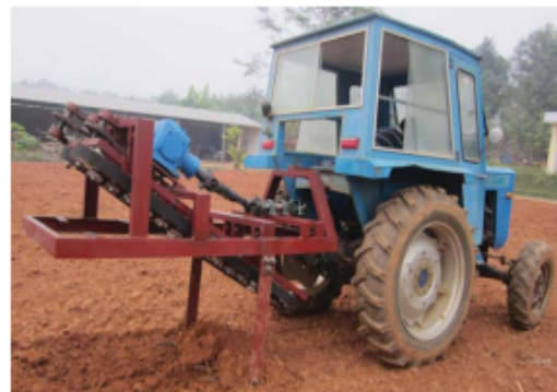
Figure 15:3-D model of digging-pulling style cassava harvester implement and cassava harvester prototype's field test(Shihao liu et al.,2014)
