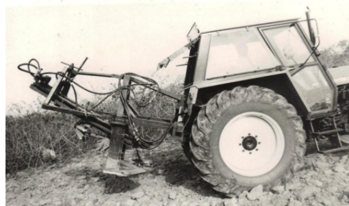
Figure 21: Leipzig mechanical cassava harvester prototype in operation (Shadrack kwadwo et al., 2011).
