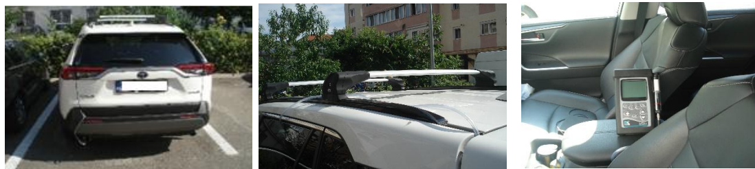
Figure 1: Toyota RAV 4 hybrid car equipped with KANE auto plus 5-1 gas analyser, ready for testing
