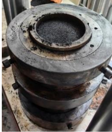
Figure12 Simulated coal sample before sampling experiment
