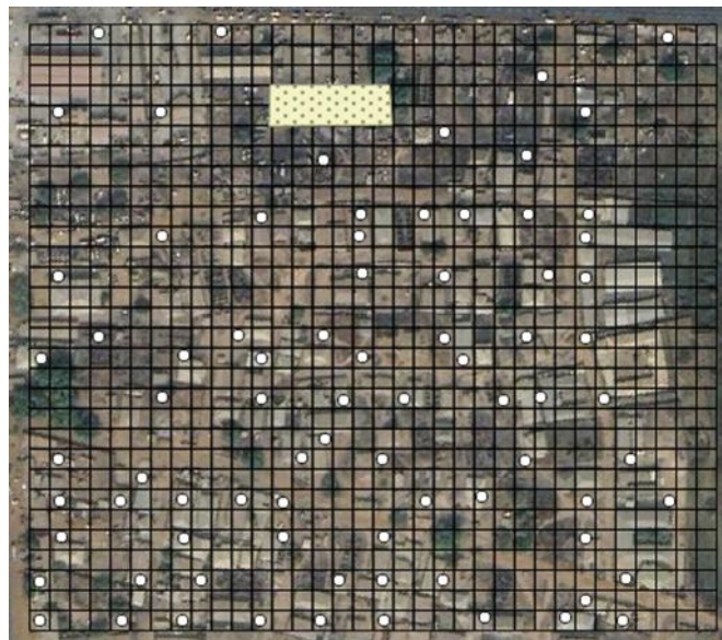
Figure 12: Representation of infiltration basins and well shapefiles
