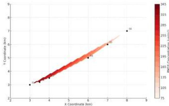
Figure 2 AERMOD PM10 plume map, confirming high concentrations around S1 and S2
