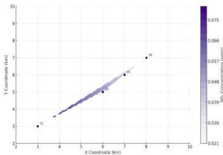
Figure 3 CALPUFF simulation for SO<sub>2</sub> dispersion up to 8 km
