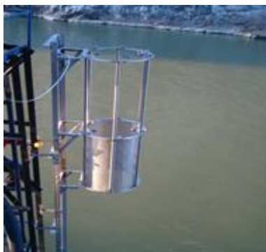
Figure 3: Submersible sensors and measuring equipment at the permanent measuring station used for real-time measurements of Vardar River water parameters
