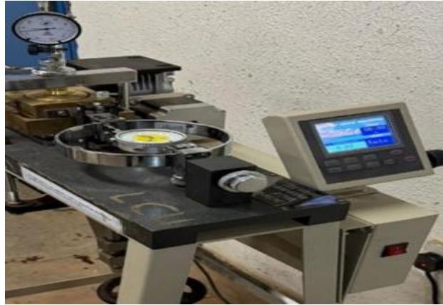
Figure 4: Determination of the cohesion of soil samples on the direct shear box
