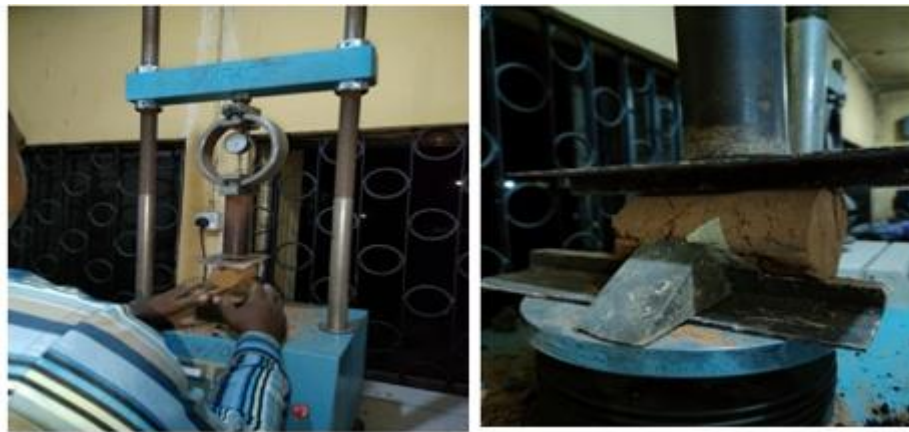
Figure 1: California Bearing Ratio (CBR) and Unconfined Compressive Strength (UCS)
