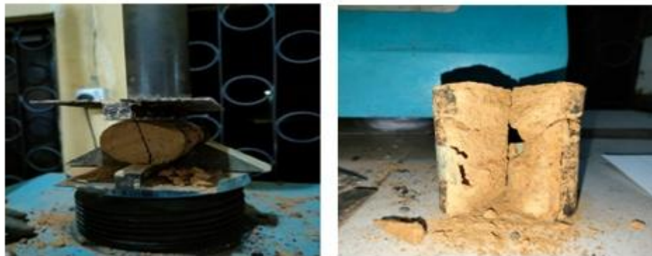
Figure 2: Indirect Tensile Strength (ITS)
