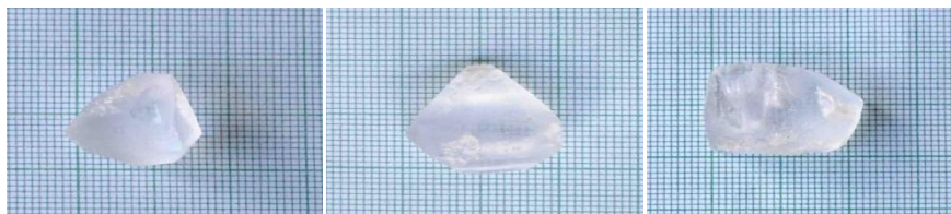
Fig.2 Photographs of the as grown pure, La-LPM and Nd-LPM crystals
