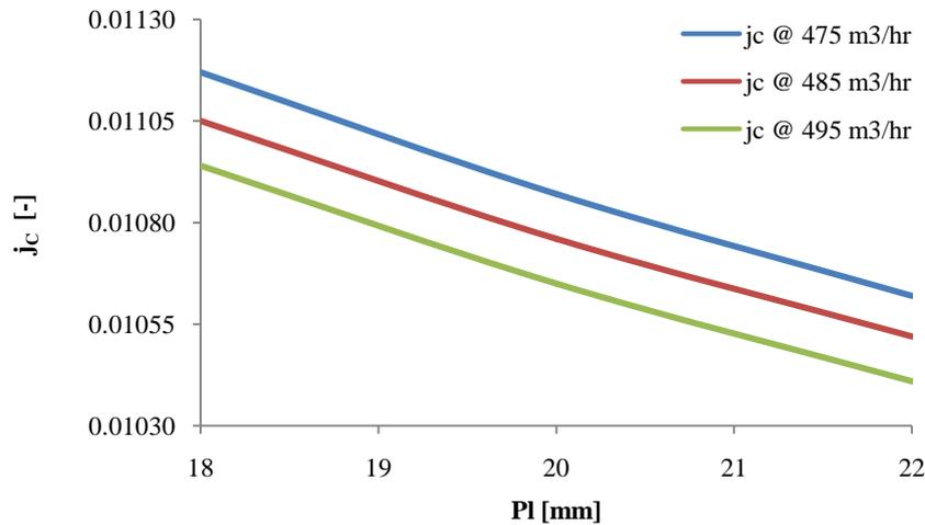
Fig. 5 Tube longitudinal pitch v/s Colburn-j factor
