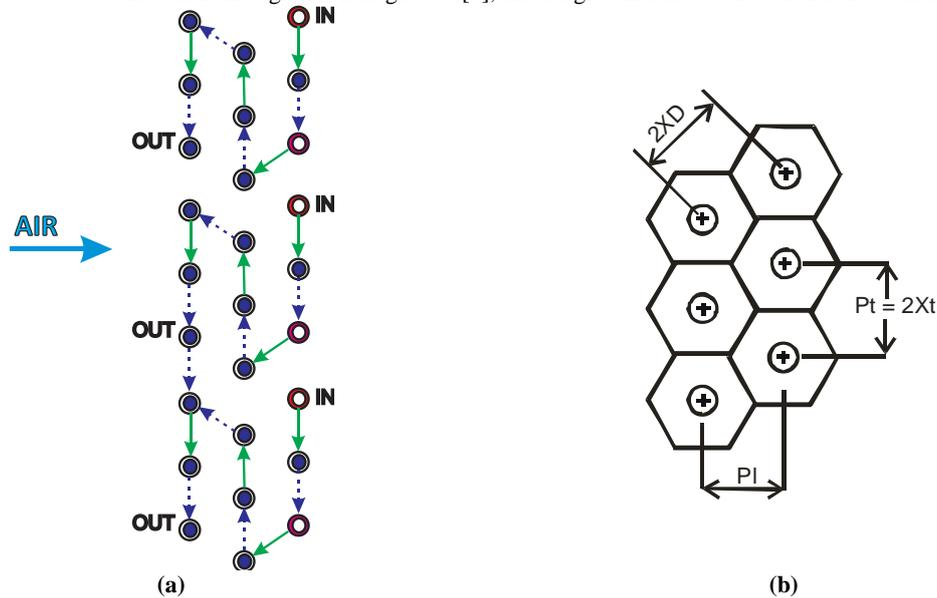
**Fig. 1** Plain-fin and tube evaporator - Staggered tube layout
