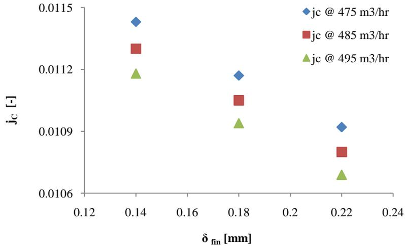
Fig. 4 Fin thickness v/s Colburn j-factor
