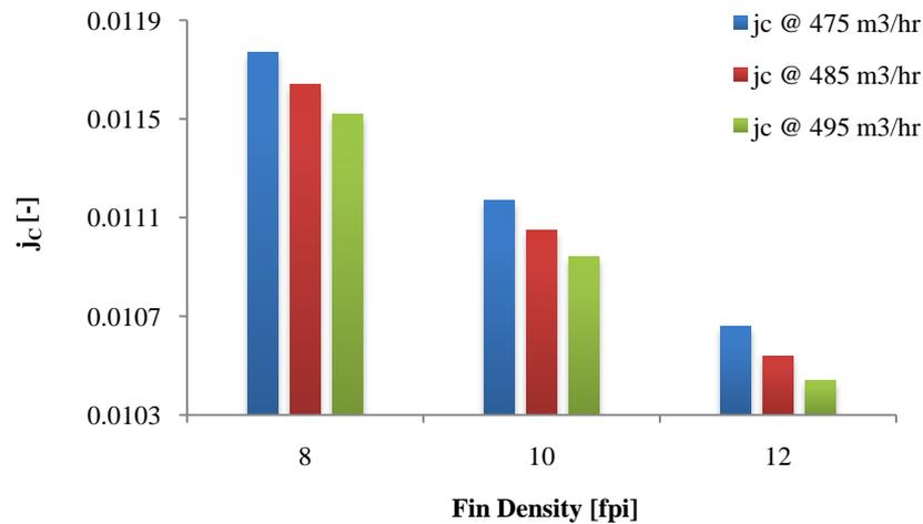
Fig. 3 Effect of fin density on Colburn j-factor
