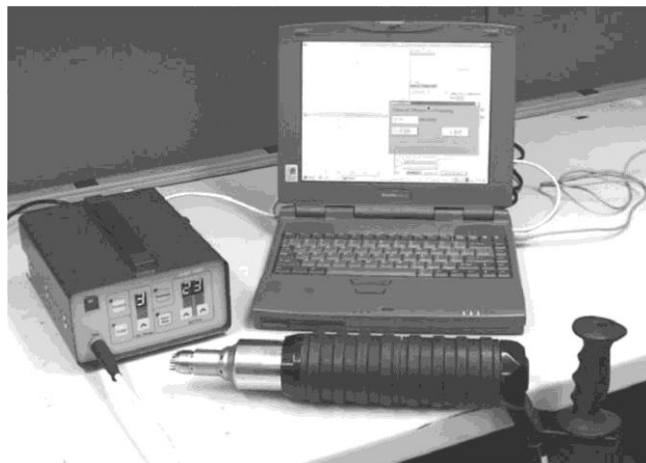
Fig. 2. A photo of the computerized complex for receiving an ultrasonic peening from (Kudryavtsev Y., Kleiman J. & Prokopenko G., 2005).
