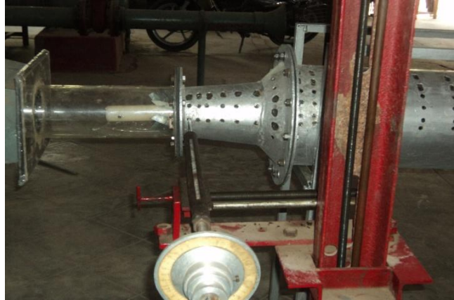
Fig.3 Experimental set up with five hole probe measurement procedure
