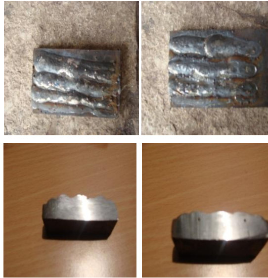
Fig : 1 showing cutting section of the hardfaced plates.
