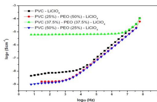
**Fig. 5:** Frequency dependence spectrum of PVC – PEO –  $\text{LiClO}_4$  system
