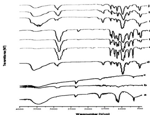
**Fig. 2:** FTIR Spectra of a) Pure PVC, b) Pure PEO, c) Pure LiClO<sub>4</sub>, d) PVC – LiClO<sub>4</sub>, e) PVC (25%) – PEO (50%), f) PVC (37.5%) – PEO (37.5%), g) PVC (50%) – PEO (25%), h) PVC (25%) – PEO (50%) – LiClO<sub>4</sub>, i) PVC (37.5%) – PEO (37.5%) – LiClO<sub>4</sub>, j) PVC (50%) – PEO (25%) – LiClO<sub>4</sub>
