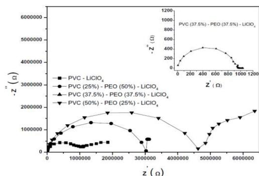
**Fig. 4:** AC Impedance Plots for a) PVC –  $\text{LiClO}_4$ ,
