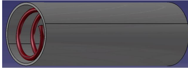
Fig.4: Heat exchanger coil
