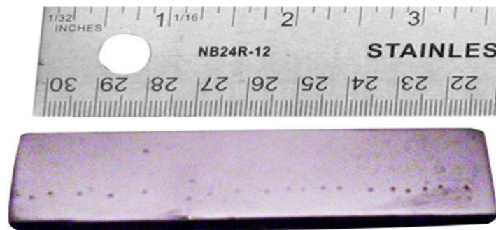
Fig.3. : Hardness test specimen.
