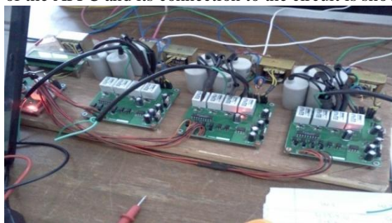
3.1 APFC with circuit connection for pf correction of an Induction motor
