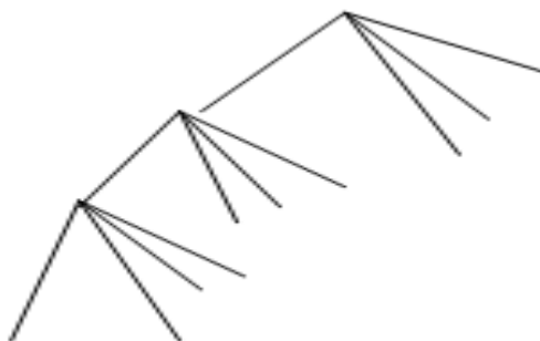
Fig1: Tree structure of wavelet decomposition
