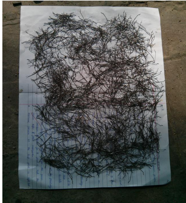
Fig: 3 Hooked End Steel Fibers used in study
